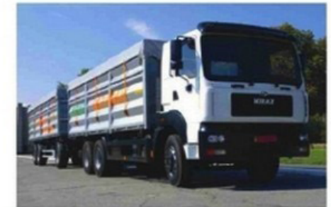
ABOVE Ukraine was once known as the breadbasket of Europe. The KrAZ-6511C4 'Caravan' grain road train has an operating gross of 46 tonnes
