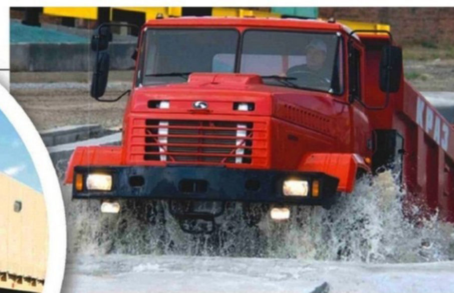
ABOVE KrAZ all-wheel drives have a wading depth in excess of one metre. This truck is being put through its paces on the company's own proving ground
