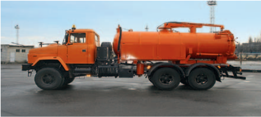
The KrAZ-6322 (KO-503IV) Sludge Pumping Vehicle Provided with Equipment from “Budshlyakhmash”
